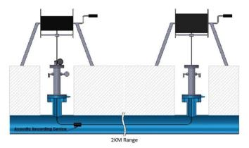
The system also records accurate distance data for leak identification to be located along the buried pipe.
