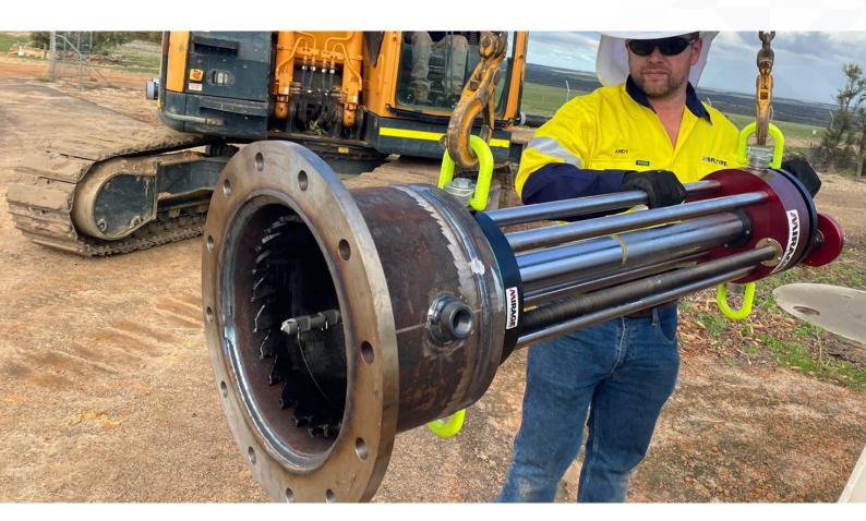
Hot Tapping is the ability to safely tie into a pressurised system while it is on stream and under pressure. It enables us to cut live tees and connections to existing water mains without the requirement for isolation of existing infrastructure. A typical Hot Tap installation consists of a tapping saddle or welded flange off take fixed to a gate valve, and Hot Tapping Machine.
